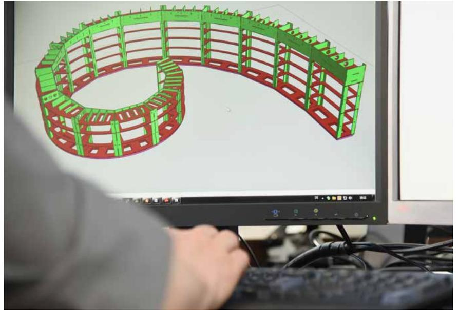
**NESTING** delivers impressive material savings while allowing a large variety of component shapes. We employ nesting in areas such as special components and furniture production, just to name two. Nesting the individual form components inside each other optimizes the consumption of raw material. This equates with less waste and greater material yield. Thanks to the use of the latest
